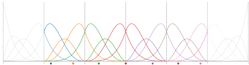
Fig. 7. Distribution of integration points: generalized Gaussian quadrature on trimmed knot vector with n_{ks} = 4 active knot spans, q = 4 and s = 1 .
