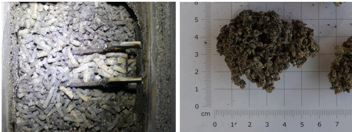
Fig. 8. Sintered ash particles after combustion of Typha ssp. in boiler 2 (left) and slag particle after combustion of Phalaris arundinacea , also from boiler 2 (right).
