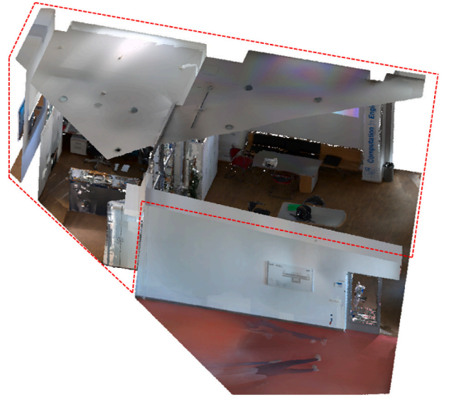
Fig. 7. Top view of visible points at camera position in Fig. 6. Points behind the wall (within the red dash line) are actually not visible from the camera pose.
