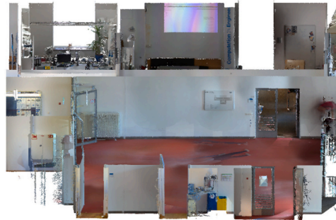
(b) Same area in laser-scanned point cloud
