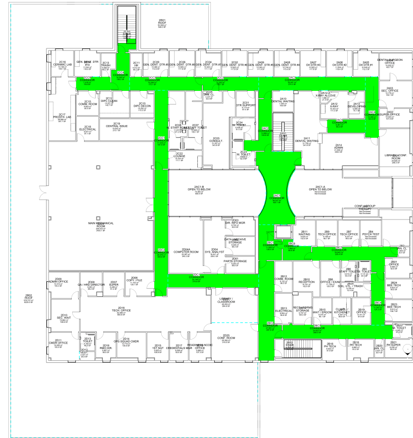
Figure 4.5: Case study model second floor circulation entities representation based on IfcSpace labels
