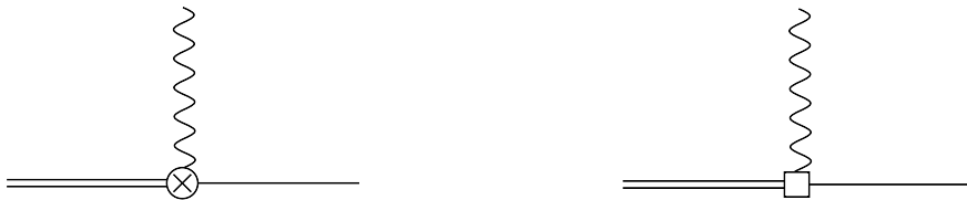
Figure 4.1: Feynman diagrams for electric and magnetic-dipole transitions between fermion-antifermion scattering states (double line) and bound states (single line). The wavy lines stand for the photon external fields. The circle with a cross denotes the electric-dipole vertex i\mathbf{r} \cdot g\mathbf{E} and the square denotes the magnetic-dipole vertex i\mathbf{r} \cdot \{\mathbf{P} \times, g\mathbf{B}\}/(4M) due to the Röntgen term [90]. The momentum \mathbf{P} is the sum of the center-of-mass momentum of the incoming fermion-antifermion pair and the momentum of the incoming photon. The vertices follow from the Lagrangian (4.2).
