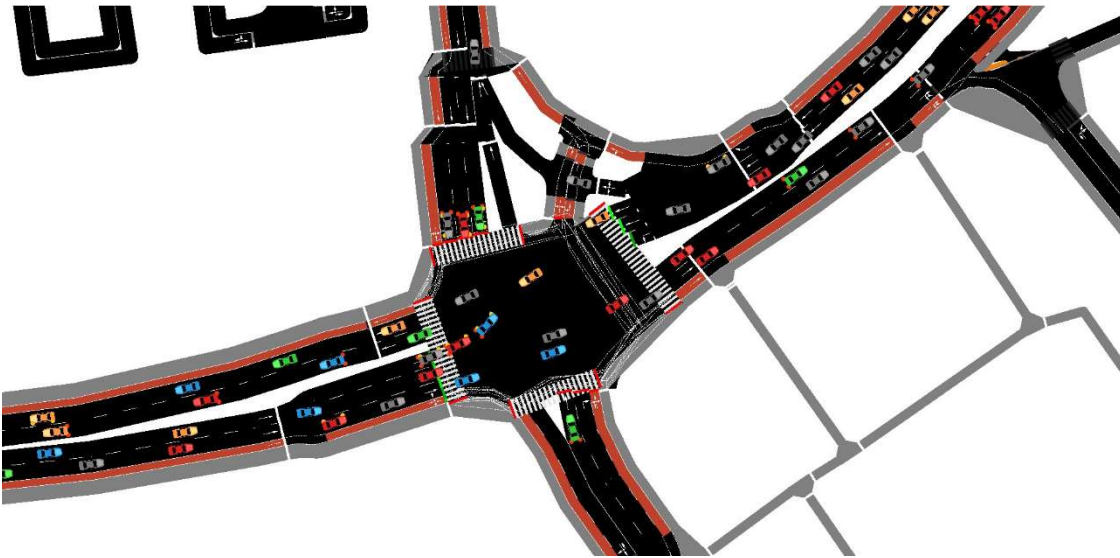
Figure 5.7: Section of the traffic model of Ingolstadt in SUMO. Automated vehicles are depicted in green, Moderate drivers in red, Speeders in grey, Timid drivers in blue and Aggressive drivers in orange.
