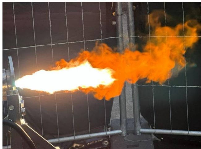
Figure 1: An arc-heated plasma torch configuration operating at 27 kW with a gas mixture of 60 SLM methane and 24 SLM hydrogen.
