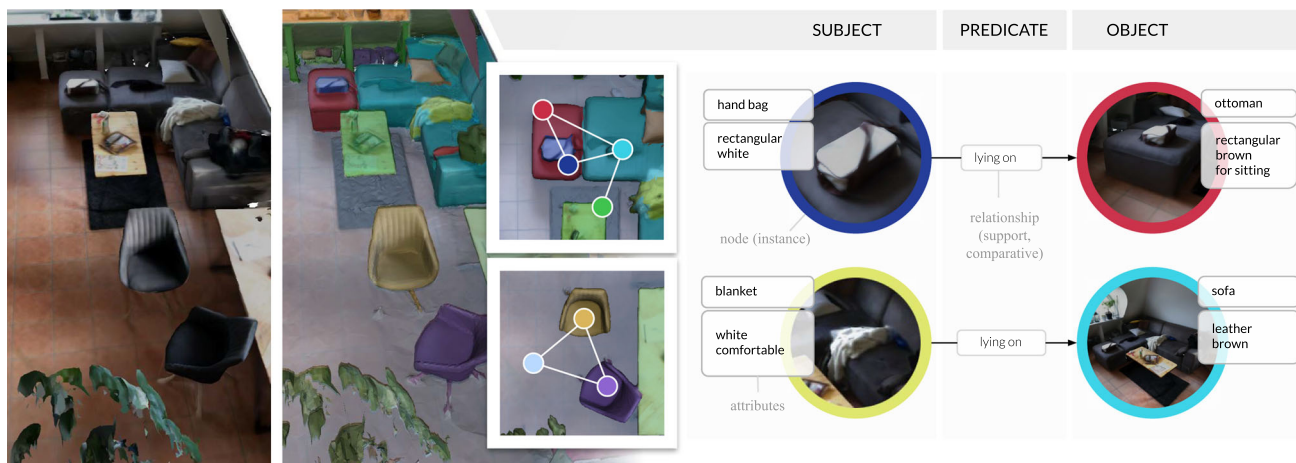
Fig. 2 Scene Graph Representation in 3DSSG consists of hierarchical class labels and attributes of scene nodes as well as semantic relationship between them. A scene graph tuple connects a subject with an object node with a predicate
