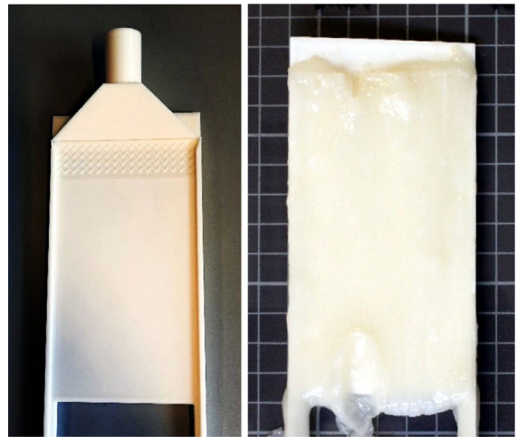
Fig. 2 Left: 3D-printed nozzle clipped onto a growth plane with a width of 6 cm and four lines of obstacles. Right: the same, overgrown with a pellicle of rheotactically oriented BC
