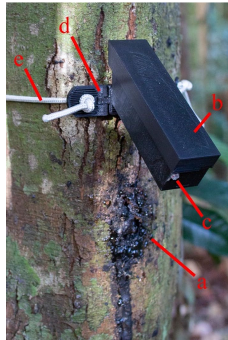
Fig. 2 Camera trap setup. a Resin wound, b camera trap, c photo-resistor, d quick release mount, and e rope around trunk
