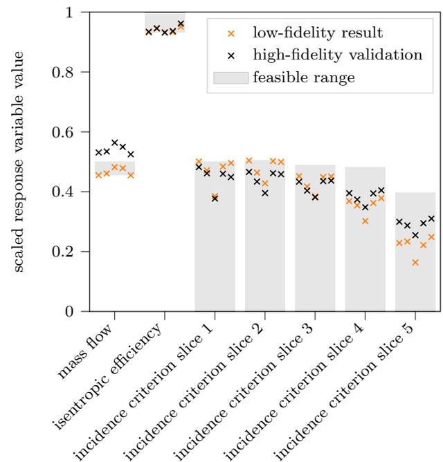
**Fig. 10** Aerodynamic response variable values for the multi-fidelity IDO results, scaled with the respective variable ranges from the sampling. The low-fidelity data-fit model results are indicated in orange, the high-fidelity CFD validations in black. The feasible ranges, that is where the optimization constraints are satisfied, are marked in light gray
