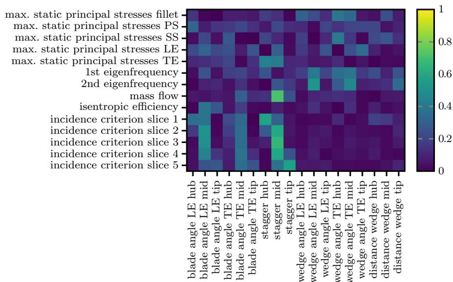
**Fig. 15** Spearman’s correlation coefficients for the design and response variables of the optimization problem defined in Table 1. The coefficients indicate a relevant monotonic relationship of the structural responses to all design variables. The aerodynamic responses show a strong correlation with blade angles and stagger in the middle of the blade, but only weakly relate to wedge angles and distance wedge
