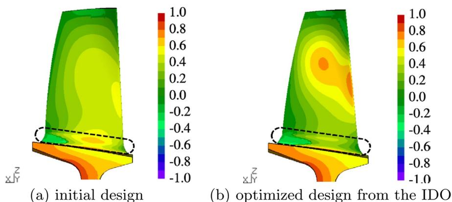
**Fig. 14** Maximum principal stress field on the rotor blade pressure side, normalized with the maximum allowed value defined in the optimization problem. In the fillet region, indicated by the dashed line, the stress peak is minimized. On the rest of the blade, the stresses stay below the maximum allowed value
