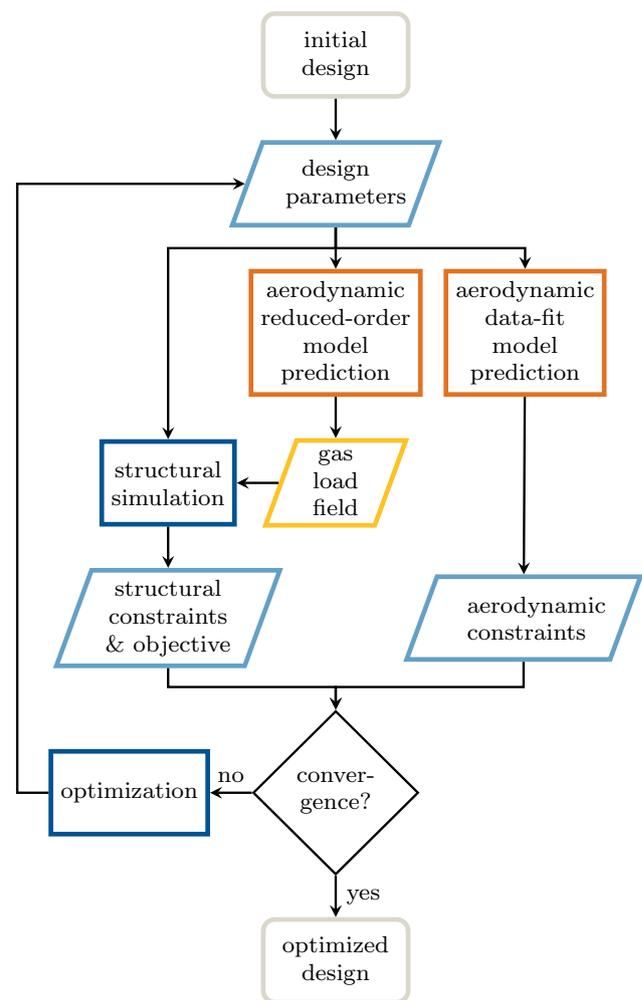
**Fig. 5** Flowchart of the proposed multi-fidelity IDO process. The structural mechanics simulations are based on high-fidelity FE models, the aerodynamic simulations are replaced by low-fidelity models
