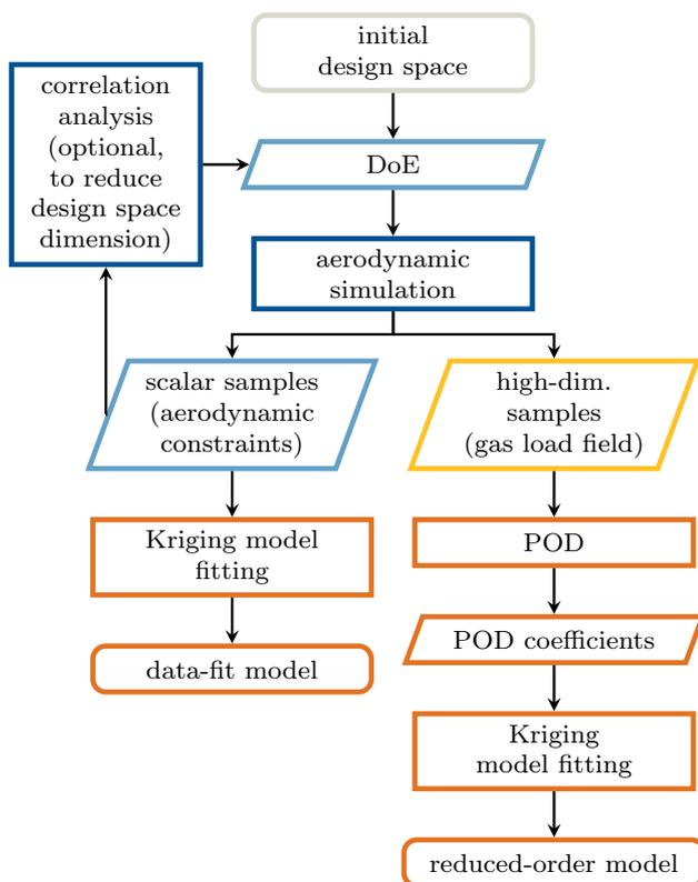
**Fig. 4** Flowchart of the low-fidelity model generation process. The high-fidelity aerodynamic model, CFD, is approximated by a data-fit model, Kriging, and a reduced-order model, consisting of POD and Kriging
