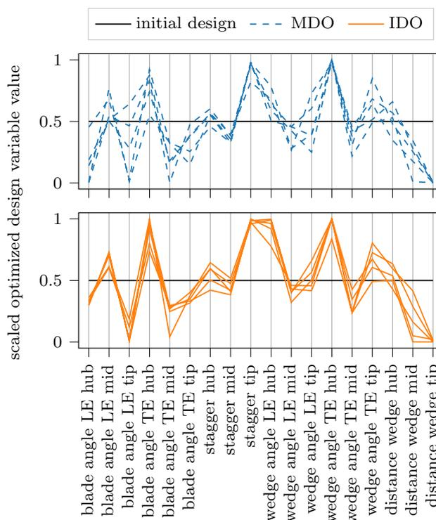
Fig. 12 Parallel coordinates plot comparing the results of the two optimization approaches to the initial design. The design variable values are scaled with their respective range
