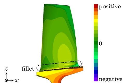
**Fig. 3** Maximum principal stress field on the rotor blade suction side as a result of the FE simulations. The stresses depend on the rotor blade geometry and are induced by centrifugal forces, thermal loads, and gas loads. The latter result from the aerodynamic pressures in Fig. 2. The dashed line indicates the fillet region
