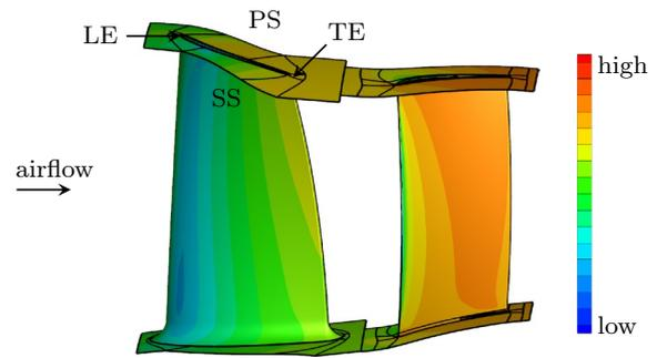
**Fig. 2** Pressure field on the third-stage rotor and stator blade surface and annulus walls as a result of the CFD simulations. The four profile sides pressure side (PS), suction side (SS), leading edge (LE), and trailing edge (TE) are indicated on the rotor blade
