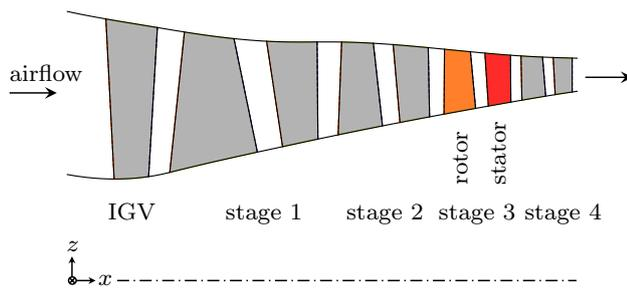
**Fig. 1** High-pressure compressor frontblock annulus geometry illustration with inlet guide vane (IGV) and four stages of rotor and stator blades. The third-stage rotor and stator blades, highlighted in orange and red, are the subject of the treated optimization problem. The arrows indicate the airflow in  $x$ -direction
