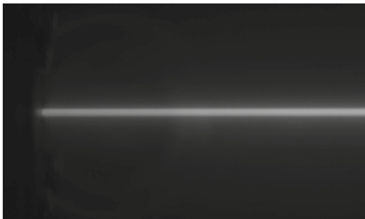
Fig. 18 Sulfur ion beam interacting with a 1 mbar argon gas target. This photograph was recorded with an ATIK383L + camera through a 740 nm Filter and the lens described in the text
