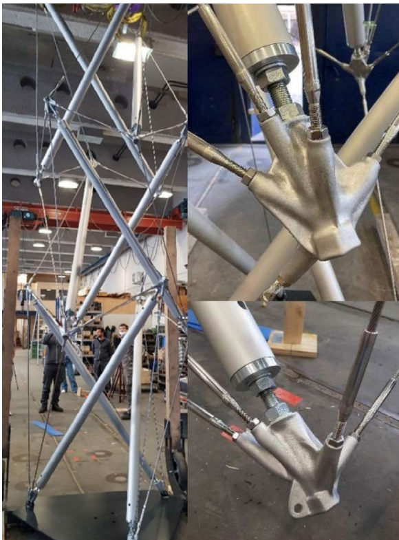
(a) The five-meter “tensegrity tower” exhibited in the Deutsches Museum of Science and Technology in Munich.
