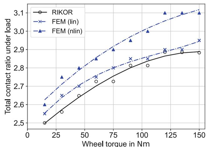
Fig. 6 Total contact ratio under load for kst-CS gear as a function of the output torque
