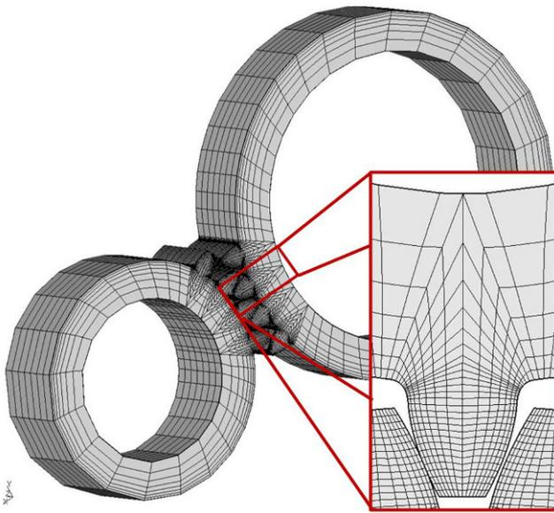
**Fig. 2** Exemplary representation of the meshing in the FE model
