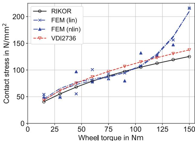
**Fig. 12** Flank pressure for kst-A gear as a function of the output torque
