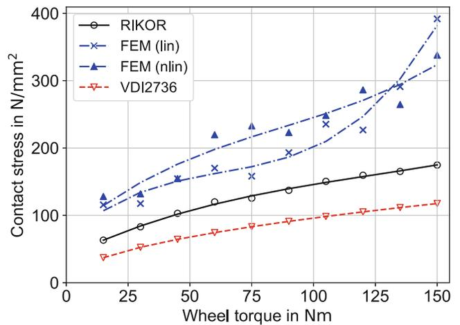
**Fig. 14** Flank pressure for kst-CS gear as a function of the output torque
