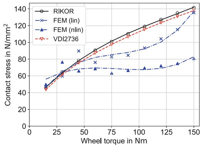
**Fig. 13** Flank pressure for kst-C gear as a function of the output torque
