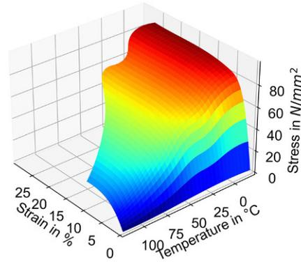
**Fig. 3** Nonlinear material model for the polymer Delrin100NC100 [31] used in the FE model
