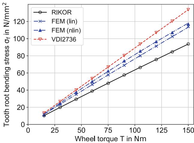
**Fig. 11** Tooth root bending stress for kst-CS gear as a function of the output torque
