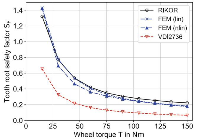
**Fig. 10** Safety factors for kst-A gear for continuous operation ( $N_L = 10^8$ ,  $S_{Fmin} = 2$ ) at 20 °C at different wheel torques
