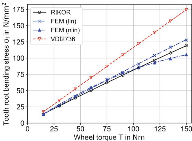
**Fig. 8** Tooth root bending stress for kst-C gear as a function of the output torque
