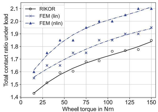
Fig. 5 Total contact ratio under load for kst-C gear as a function of the output torque
