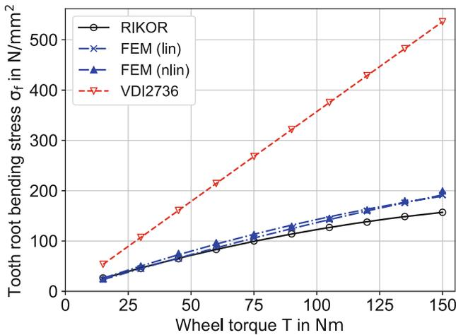
**Fig. 7** Tooth root bending stress for kst-A gear as a function of the output torque
