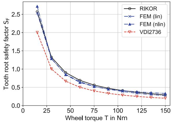
**Fig. 9** Safety factors for kst-C gear for continuous operation ( $N_L = 10^8$ ,  $S_{Fmin} = 2$ ) at 20 °C at different wheel torques
