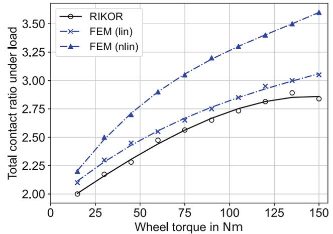
Fig. 4 Total contact ratio under load for kst-A gear as a function of the output torque
