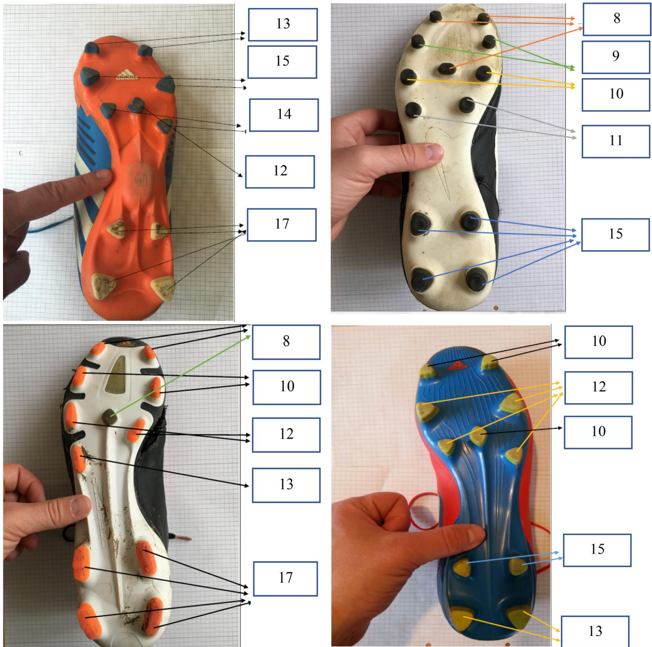
Fig. 3 Photographs of four outsoles of football boots measured their stud heights used in Data base (all dimension in mm)
