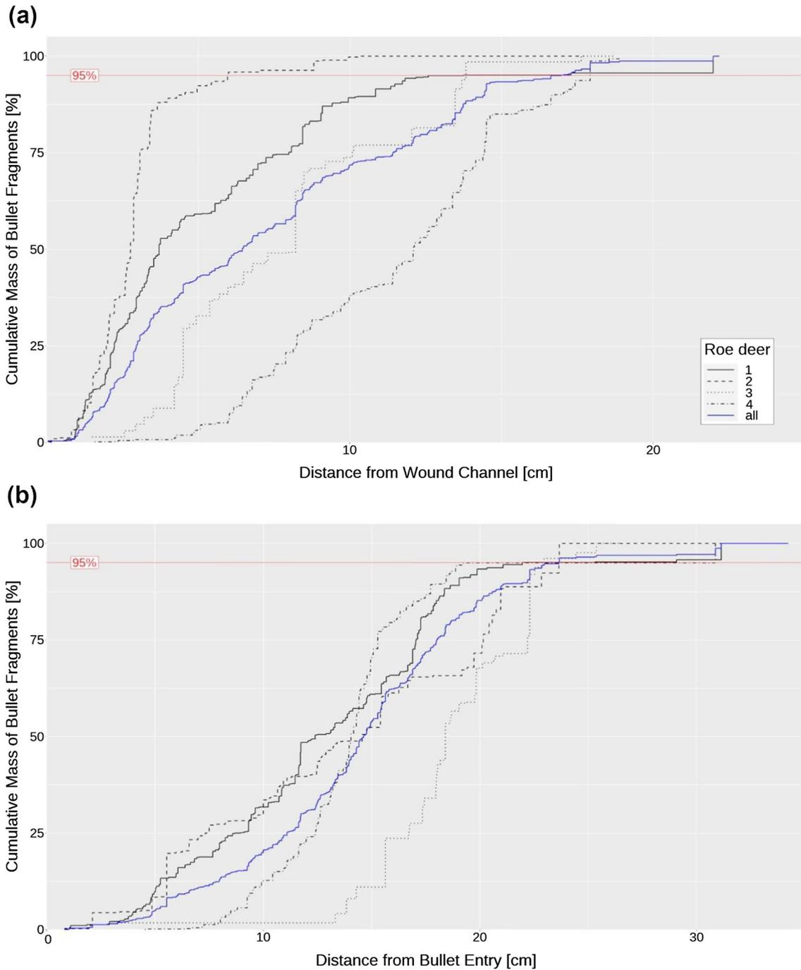
**Fig. 5** Cumulative bullet fragment mass (BFM) in relation to the **a** perpendicular distance (radius) from the wound channel and **b** in distance to the bullet entry for the four roe deer bodies (A.0)
