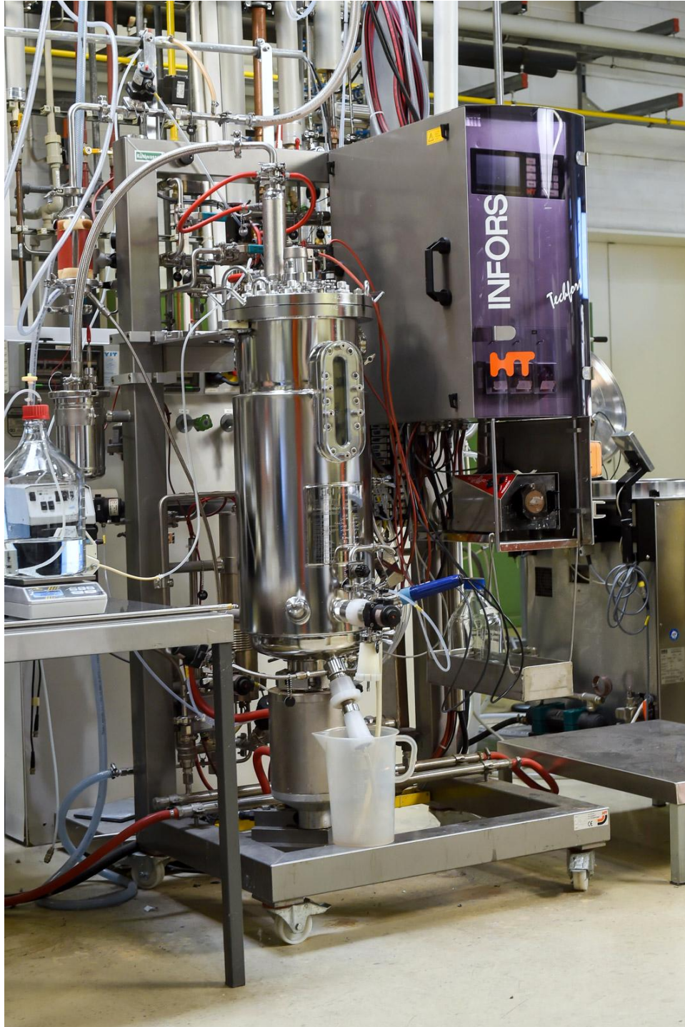
Figure 4.3: Stirred-tank bioreactor for cultivation experiments on the 25 L scale (Photo: Tobias Haase, TUM).
