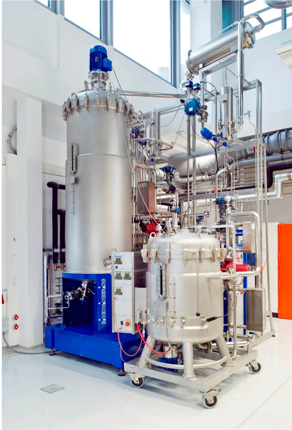
Figure 4.5: Stirred-tank bioreactor for cultivation experiments on the 1000 L scale (Photo: Andreas Heddergott, TUM).
