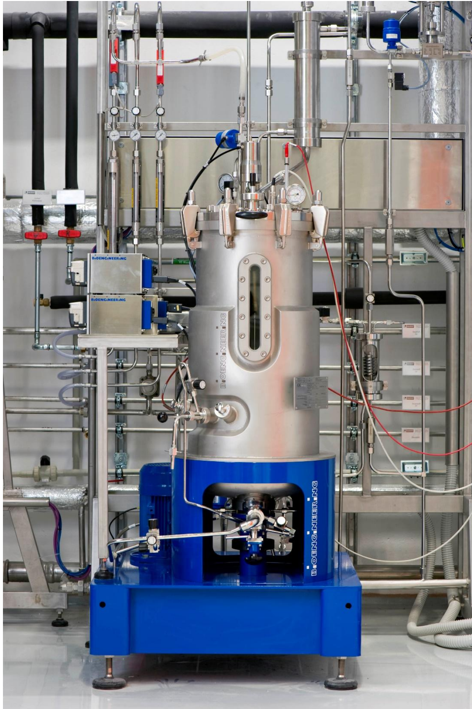
Figure 4.4: Stirred-tank bioreactor for preculture preparation of A. niger NRRL 2270 (Photo: Andreas Heddergott, TUM).
