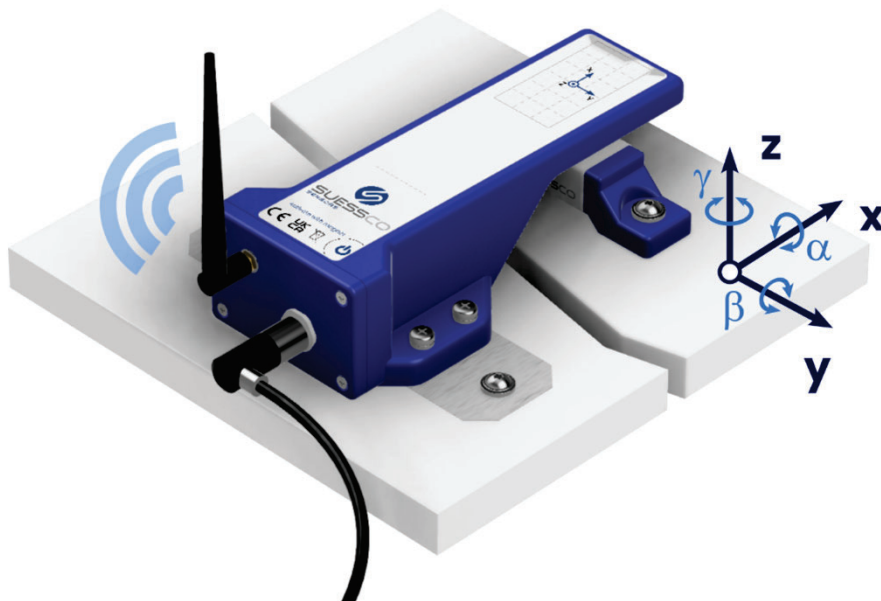
Figure 1: 6D position sensor based on magnetic field measurements showing axis orientation.
