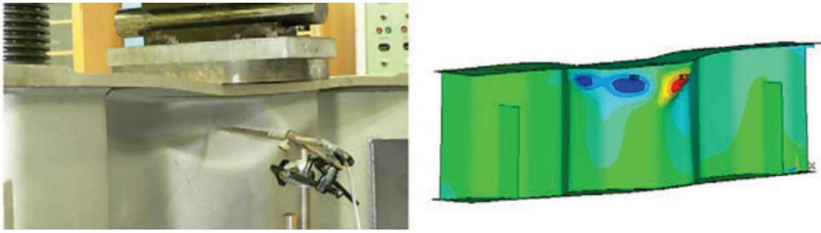
Figure 4: Experimental and numerical investigations on patch loading resistance.
