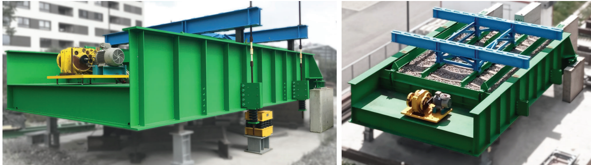
Figure 8: Large-scale test facility for targeted and isolated research of energy dissipation mechanisms in ballasted track under dynamic excitation and for isolated research of the dynamic properties of the longitudinal track-bridge interaction
