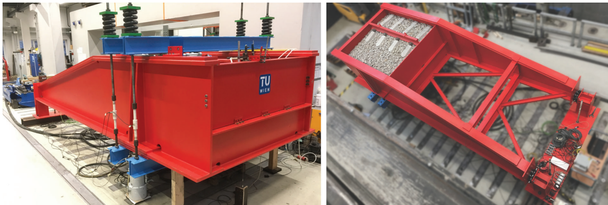
Figure 9: Large-scale test facility for targeted and isolated research of vertical energy dissipation in ballasted track and dynamic properties of the vertical track-bridge interaction
