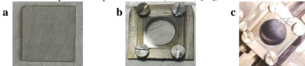
Fig. 10A.2. HVPE free-standing Ga polar Si-doped GaN (0001) and N polar Ge-doped GaN (000 \bar{1} ). (a) A sample before mounting on a holder. (b) A sample after mounting on the JT-STM holder and before any cleaning cycle. (c) A sample on the holder of JT-STM after the
