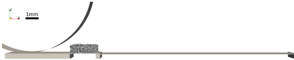
Fig. 1. Simulation setup with roller, fully extended powder reservoir piston with 42,000 particles and powder reservoir.
