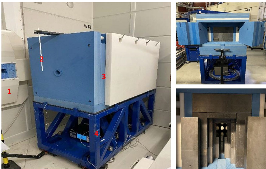
Fig. 1 The left picture shows the FaNGaS spectrometer with the upgraded shielding at experimental position: 1 front side of the new MEDAPP multi-leaf neutron beam collimator; 2 holder for small samples made of Teflon; 3 HPGe-detector shielding; 4 iron support
