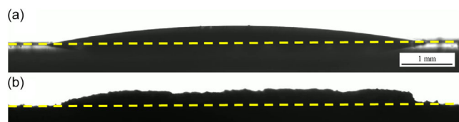
Figure 10. Image captured 5 minutes after the initiation of the melting process on a Haynes 214 substrate: a) BNi-5 filler and b) CCA filler. The yellow dashed lines indicate the baselines for the contact angle measurements.
