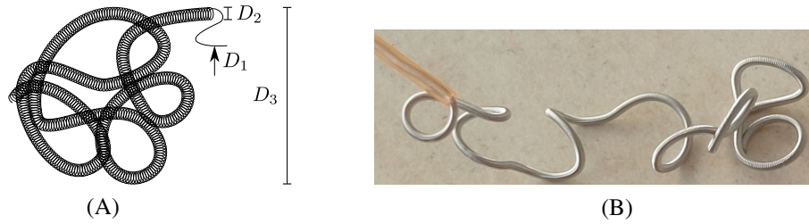
FIGURE 6 Sketch and photo of coiling wires. (A) Schematic micro structure of a coiling wire: D_3 denotes the approximate diameter of the coil-node forming within the aneurysm, D_2 the apparent diameter of the (macroscopic) coiling wire and D_1 the diameter of the actually microscopic wire wrapped in a helical way to form the macroscopic ( D_2 ) wire. (B) Expulsion of an actual coil into regular surrounding (air) with contactless loop formation and curling.
