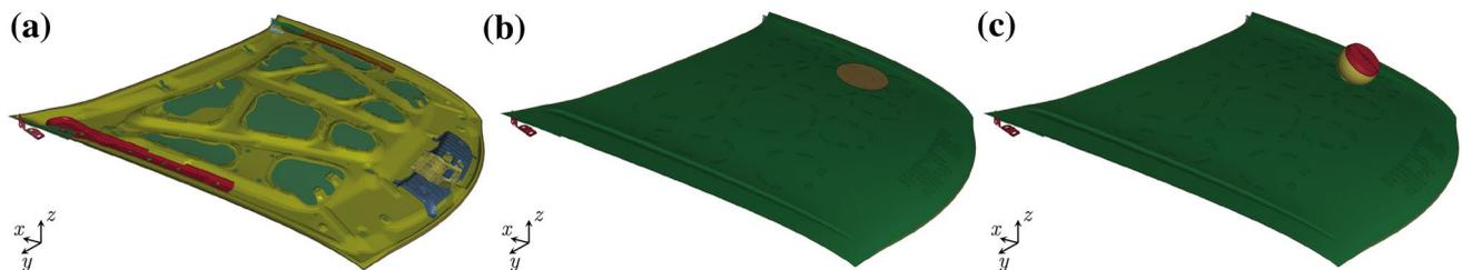
**Fig. 16** Setup of the pedestrian safety load cases. Detailed (partially transparent) depiction of the used hood of the Honda Accord FE model (a) [42], simplified simulation setup using concentrated nodal
