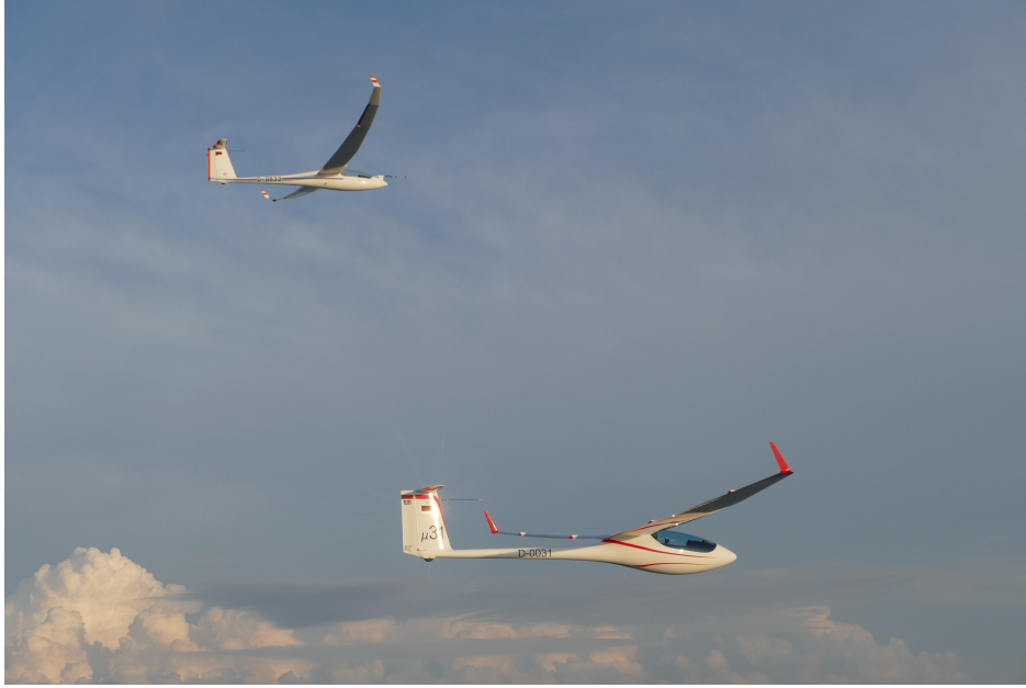
Figure 6.1: Photograph of side-by-side flight performance measurement of the Mü31 comparison sailplane. Reference sailplane Discus 2c DLR in background
