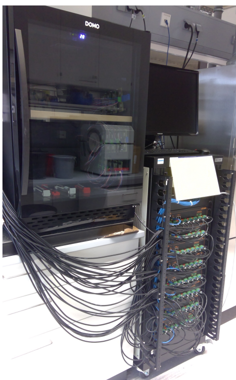
Figure S7: The hardware setup of the cyclor used in this study including the control unit on the right and the temperature chamber on the left.
