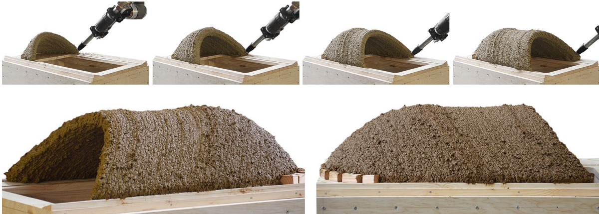
Figure 6: Design study No.11. Top: fabrication of the cap. Starting from P_p of 25%, every picture shows 25% steps up to the final print on the right side. Bottom: cap after fabrication.
