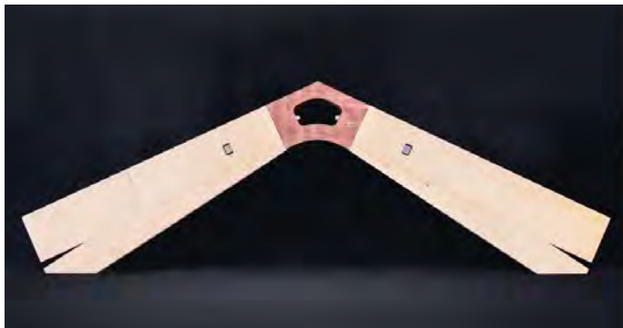
Bild 12 Mock-up (M 1:1) des reversiblen Firstknotens Mock-up (scale 1:1) of the reversible ridge knot
