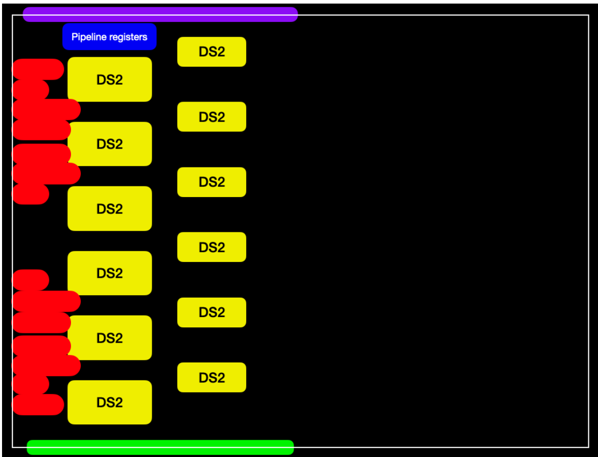
Figure 2.5.: Semi-interleaved memory-buffer stages floorplan
