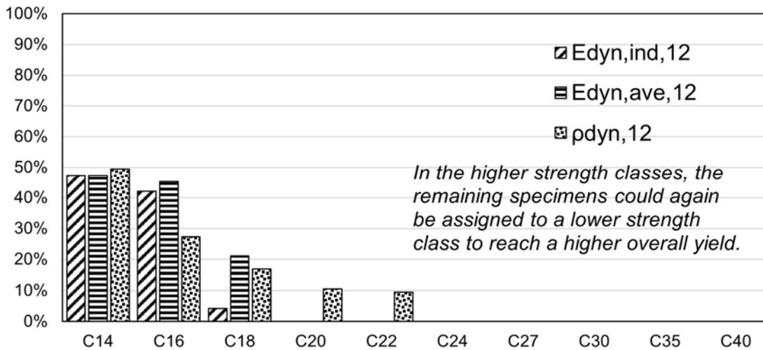
Figure 30: Yield per bending strength class based on the machine grading
