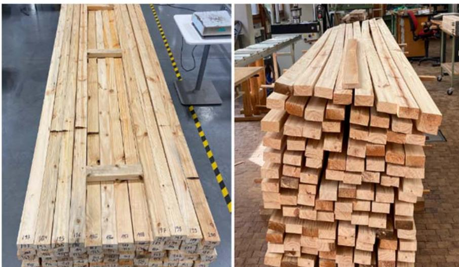
Figure 4: Deformations of the specimen (warping) due to changes in moisture content before storage at standard climate (left) and after storage in standard climate (right) (Simon Kramer)
