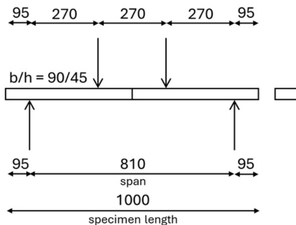
Figure 9: Test setup and dimensions of the bending test specimens with finger joints in [mm]
