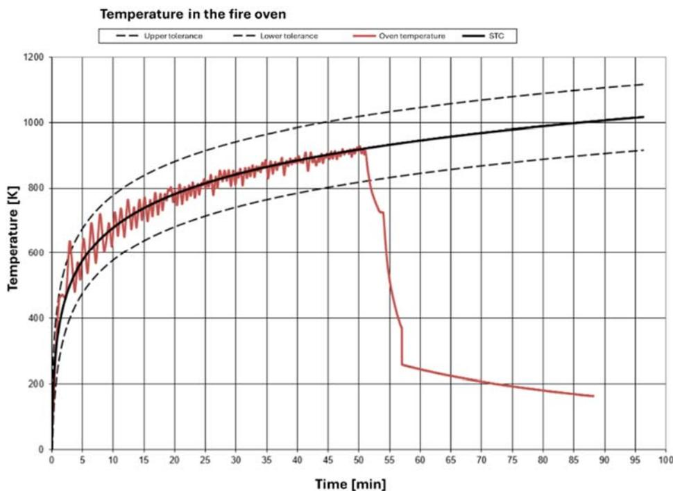
Figure 17: Temperature-time-curve of one of the fire tests
