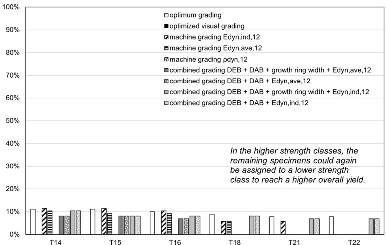
Figure 26: Comparison of the yield of the different grading methods for strength classes T14 to T22
