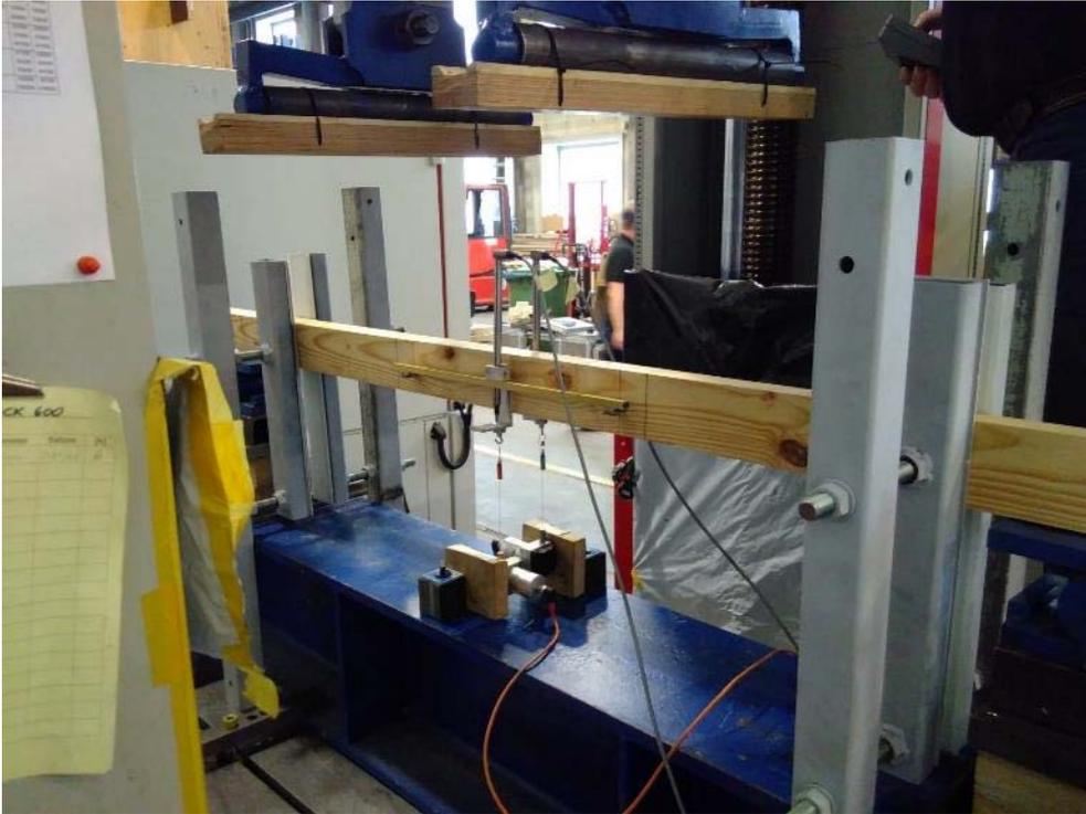
Figure 8: Test setup for the bending tests in the laboratory (Lucas Viereck)
