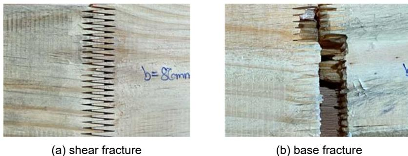
Figure 35: Fracture modes of the finger joints tested in bending (Simon Kramer)
