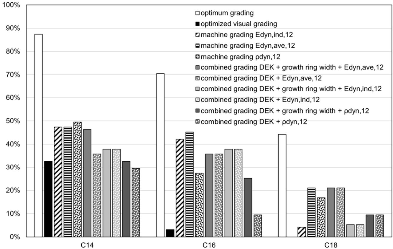
Figure 32: Comparison of the yield of the different grading methods for strength classes C14 to C18
