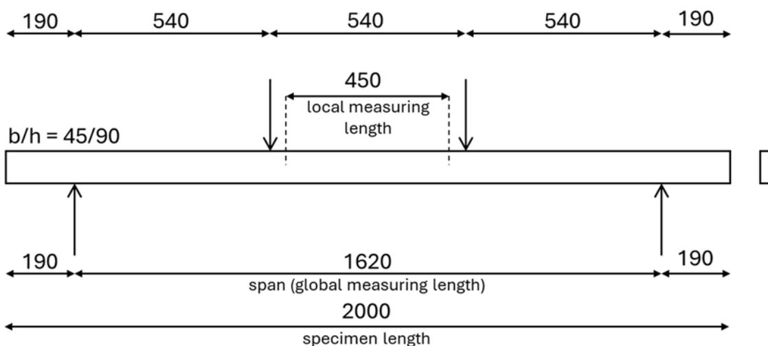
Figure 7: Test setup and dimensions of the bending test specimens in [mm]
