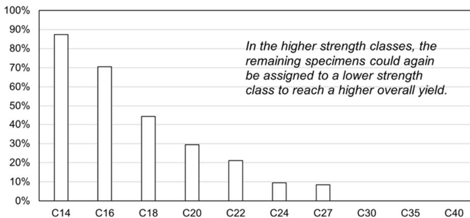
Figure 28: Maximum possible yield per bending strength class based on the optimum grading
