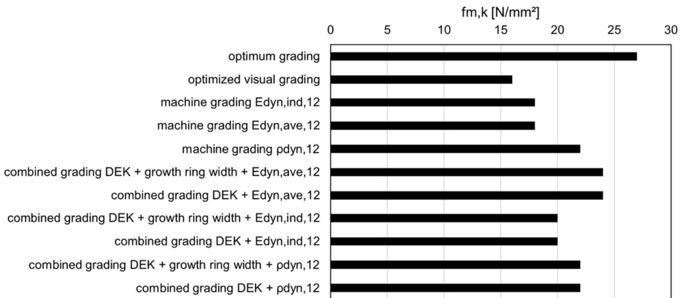
Figure 34: Maximum strength class that the different grading methods can reach
