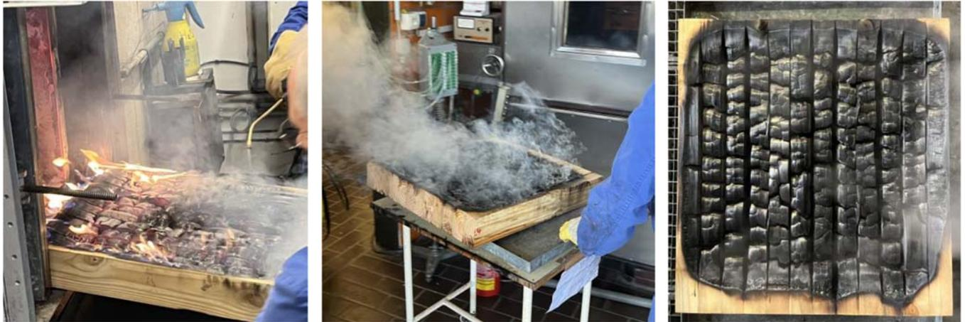
Figure 18: Removal of a fire test specimen from the oven (Nicole Ebert)
