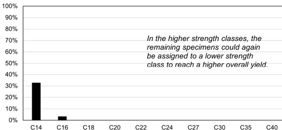
Figure 29: Yield per bending strength class based on the optimized visual grading
