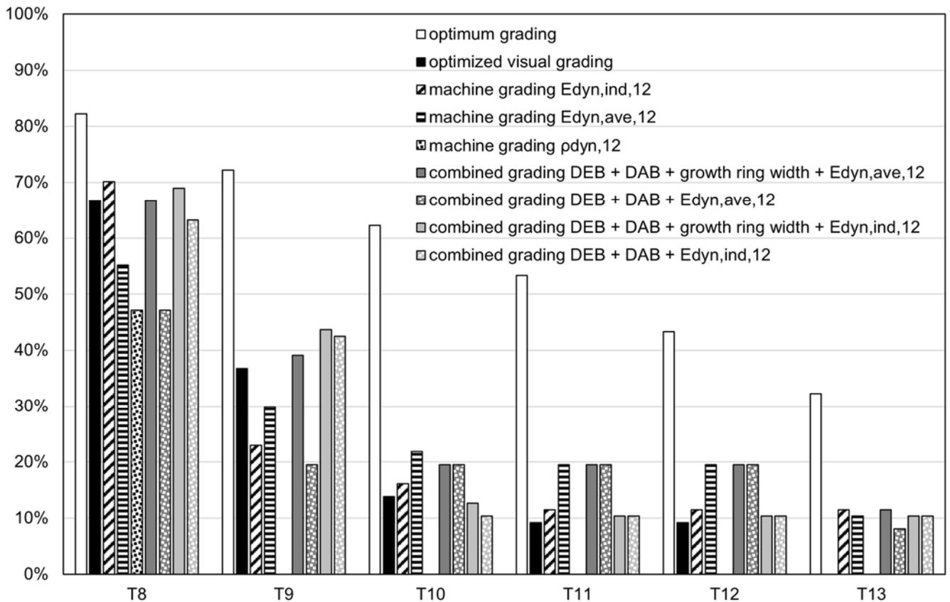
Figure 25: Comparison of the yield of the different grading methods for strength classes T8 to T13
