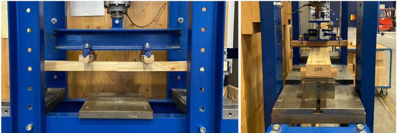
Figure 10: Test setup for the bending tests on finger joints in the laboratory (Simon Kramer)
