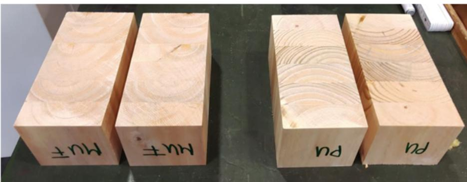
Figure 13: Finished delamination specimens (Nicole Ebert)
