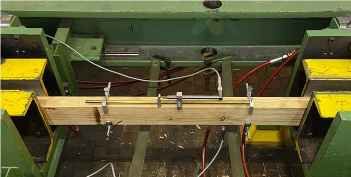
Figure 6: Test setup for the tensile tests in the laboratory (Simon Kramer)
