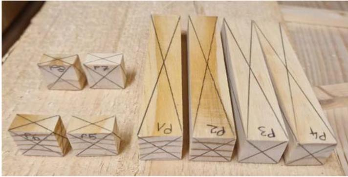
Figure 20: Specimens for the measurement of the swelling and shrinkage – left: specimens for the radial and tangential measurement, right: specimens for the longitudinal measurement (Nicole Ebert)
