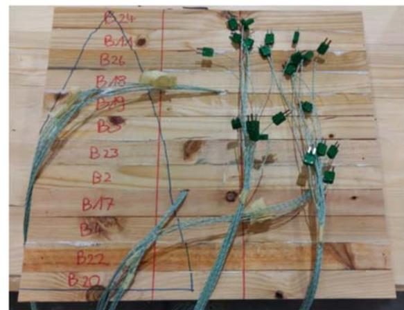
Figure 15: Finished fire test specimen with integrated thermocouples (Nicole Ebert)
