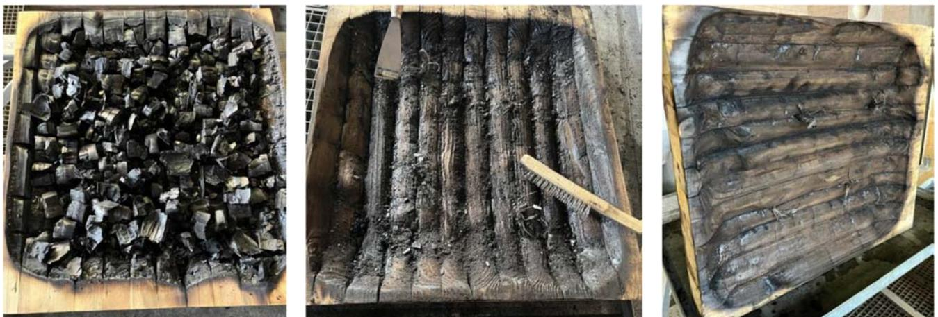
Figure 19: Removal of the coals from a fire test specimen (Nicole Ebert)
