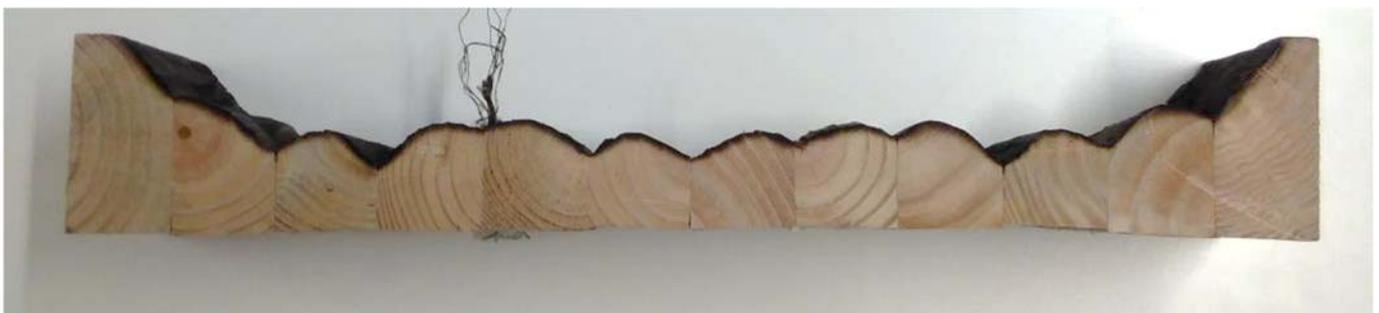
Figure 36: cross-section of a fire test specimen after the test (Lucas Viereck)
