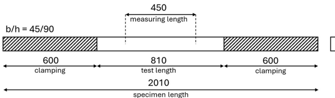
Figure 5: Test setup and dimensions of the tensile test specimens in [mm]
