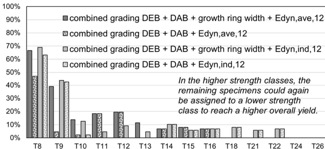
Figure 24: Yield per tensile strength class based on the combined visual and machine grading
