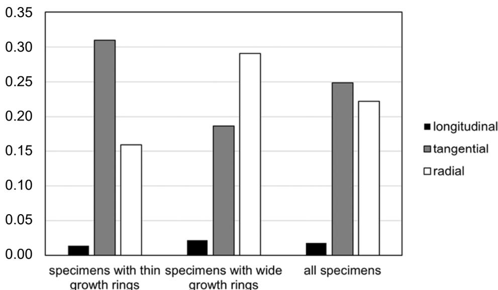
Figure 37: Differential swelling parameters
