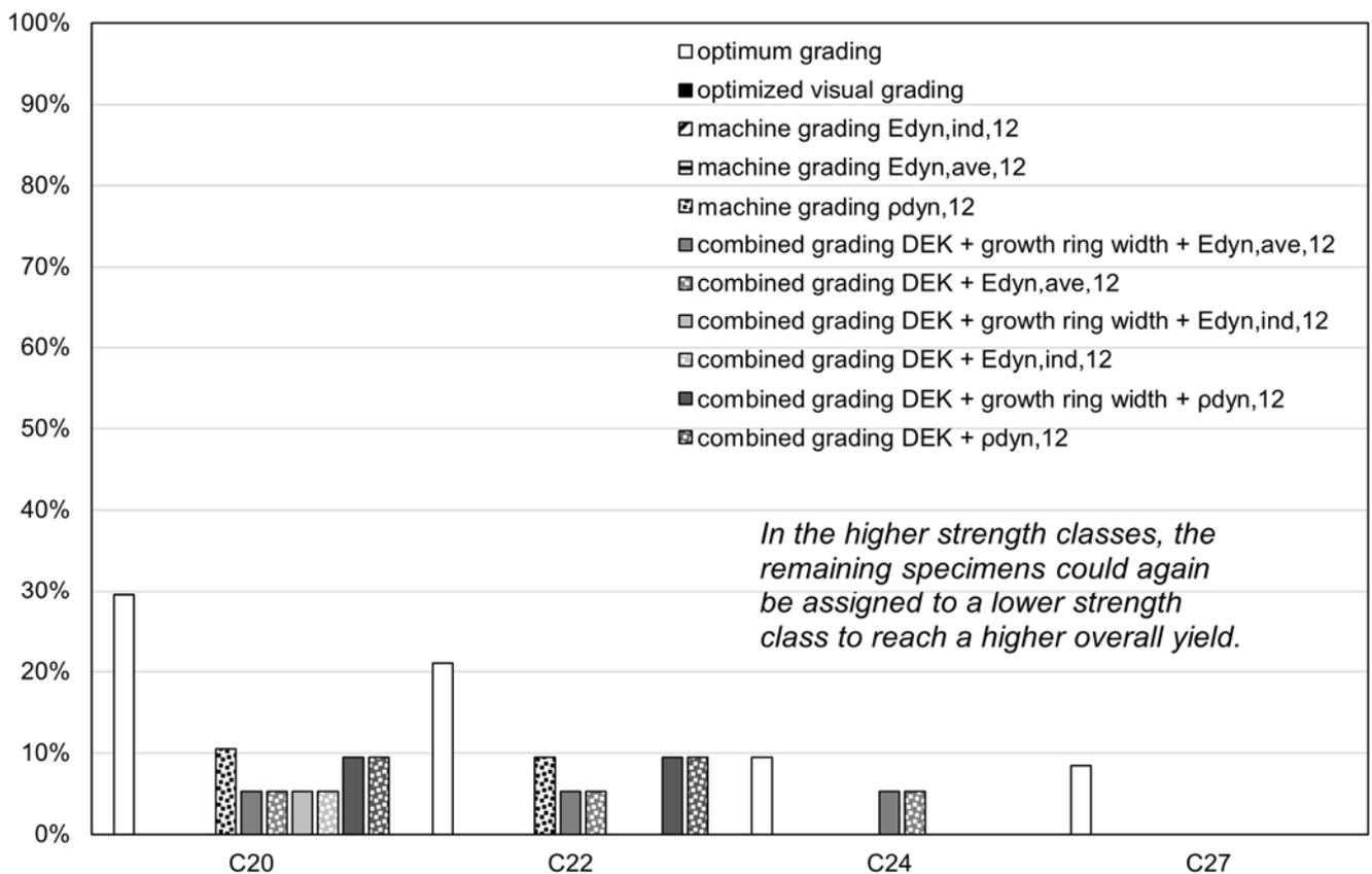
Figure 33: Comparison of the yield of the different grading methods for strength classes C20 to C27
