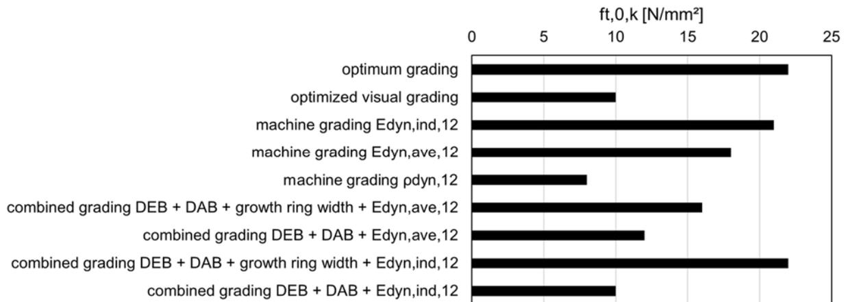
Figure 27: Maximum strength class that the different grading methods can reach
