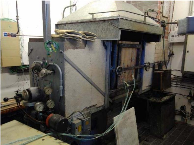
Figure 16: Small fire oven with installed test specimen at its side (Lucas Viereck)
