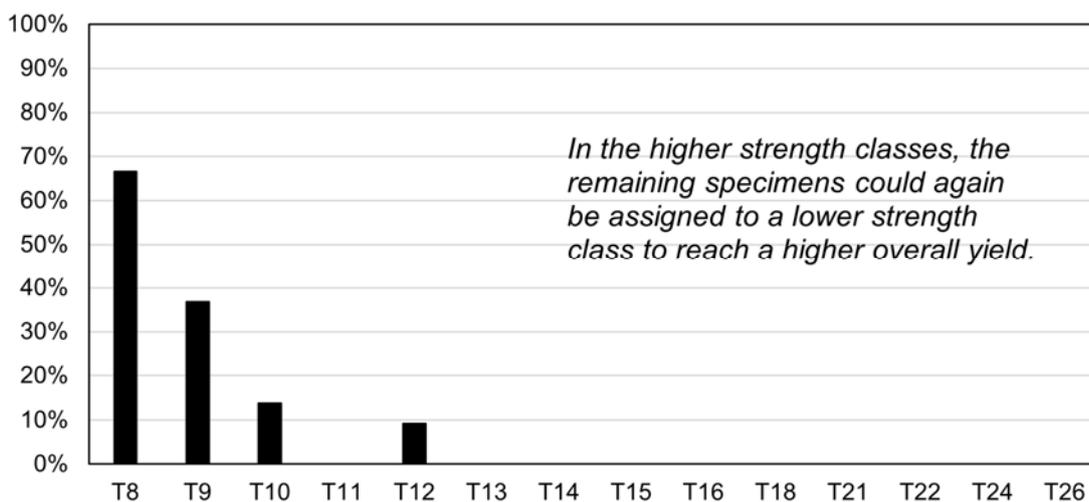
Figure 22: Yield per tensile strength class based on the optimized visual grading
