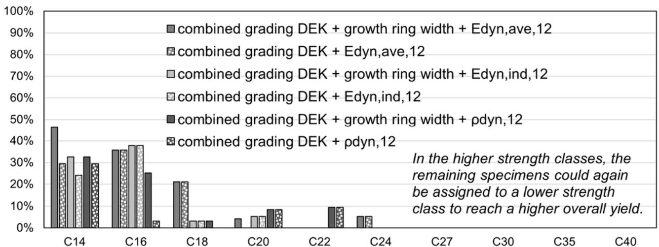
Figure 31: Yield per bending strength class based on the combined visual and machine grading
