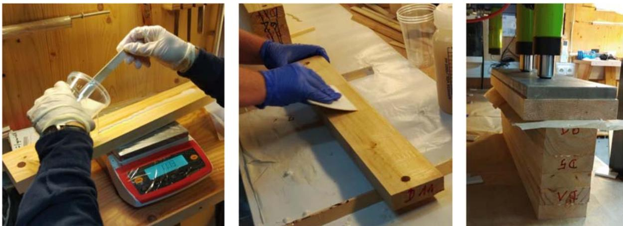
Figure 12: Gluing of the delamination specimens (Nicole Ebert)
