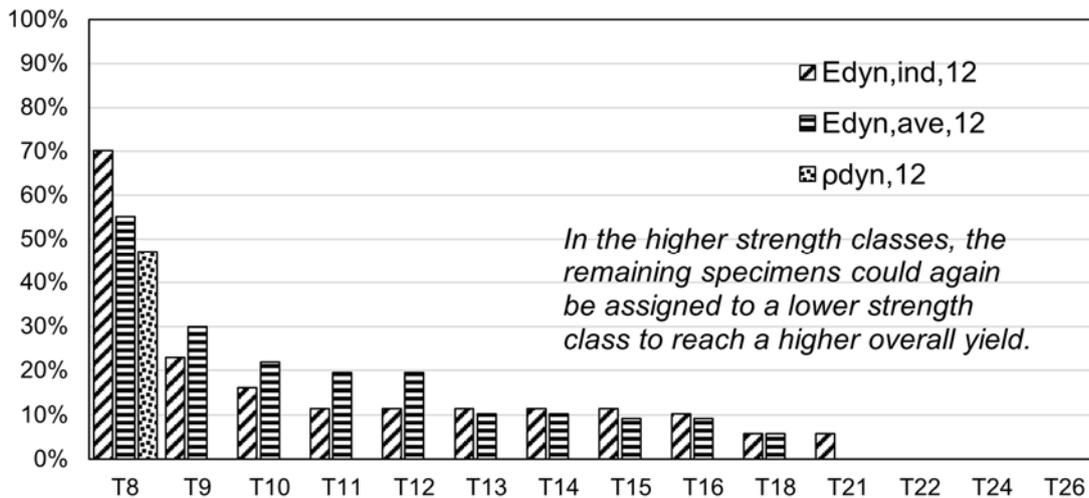
Figure 23: yield per tensile strength class based on the machine grading
