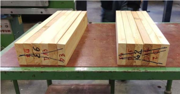
Figure 11: Samples for the preparation of the delamination specimens (Nicole Ebert)
