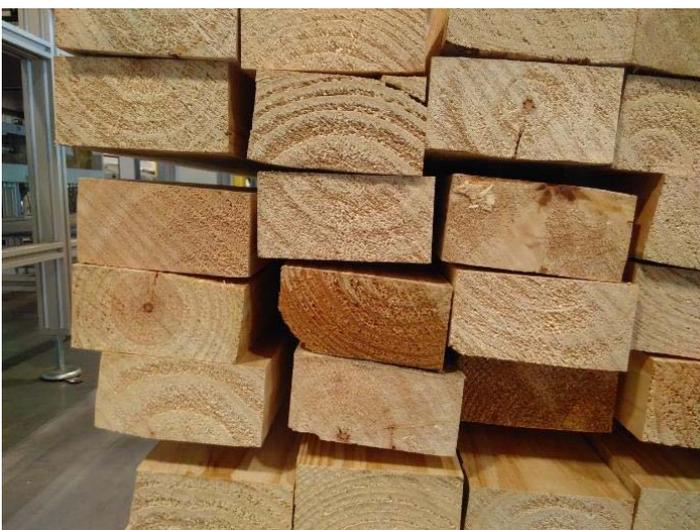
Figure 2: Timber cross-sections of *pinus patula* with characteristic wide growth rings
