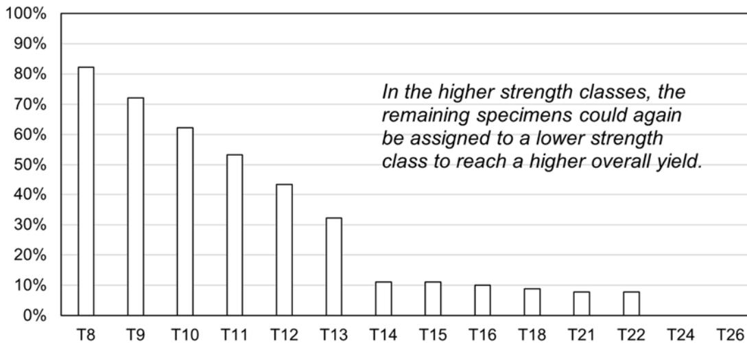
Figure 21: Maximum possible yield per tensile strength class based on the optimum grading
