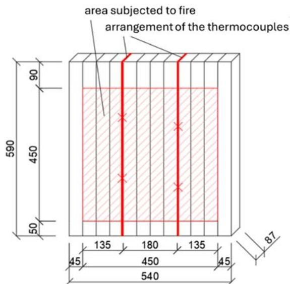
Figure 14: Drawing of the fire test specimens (Nicole Ebert)
