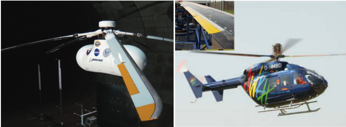
(a) Boeing SMART rotor with active trailing-edge flaps in the NASA Ames wind tunnel [41]. (b) First flight of the BK117 helicopter with active trailing edge flaps [100].
