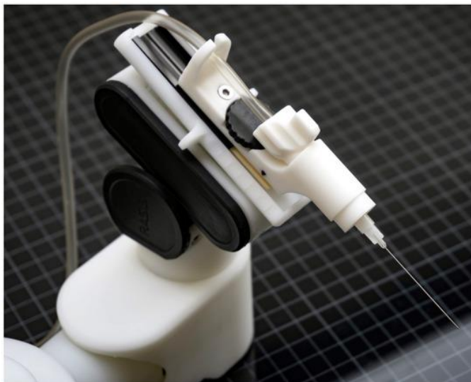
Illustration 6: Custom-made robot holding injection cannula.
