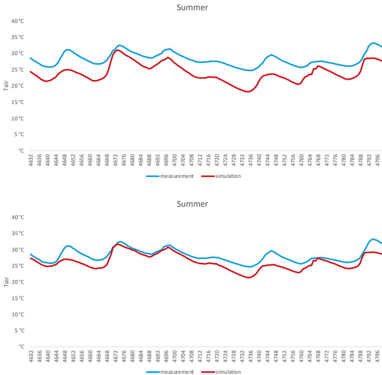
Figure 3-6: Curve for the simulated (red) and the measured (blue) air temperature for the summer before (top) and after (low) validation (own representation based on calculations acc. to [3-10])
