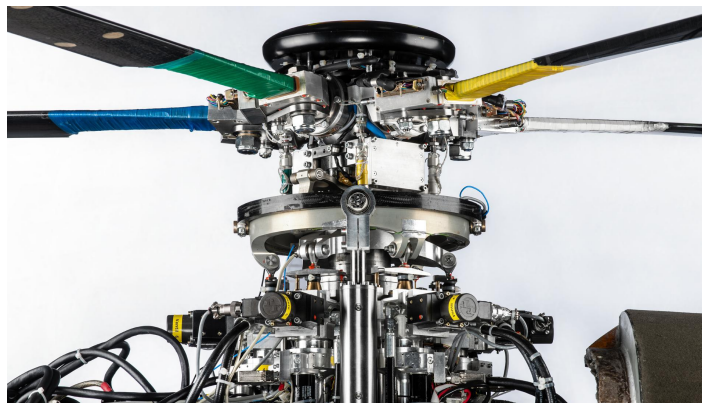
Figure 1.1.: The META rotor system from DLR for individual blade control via passive pitch links[1](CC BY-NC-ND 3.0 DEED).
