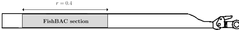
Figure 2.18.: Illustration of the active camber morphing section modeled on the Bo 105 rotor blade.
