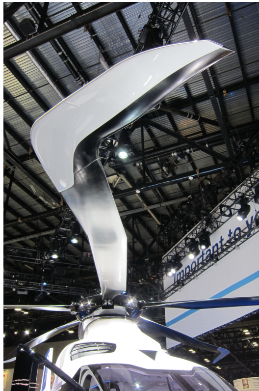
Figure 1.9.: Blue Edge rotor blade for passive noise reduction [14]. Photo taken by Nick Isaacs [CC BY-SA 4.0 DEED].
