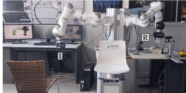
Fig. 5: Setup of the teleoperation station with haptic input device [I] on the left and remote robot on the right [R].
