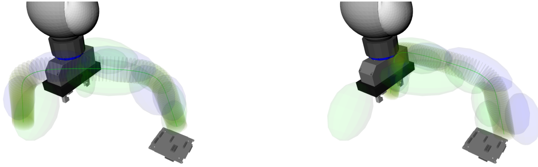
(1) Original task-parametrized trajectory not starting from the (2) Modified trajectory starting from the current end effector pose.
