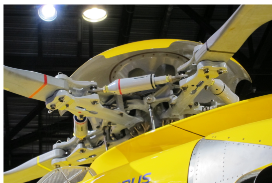
(a) Airbus Helicopters H175 rotor head [91].
