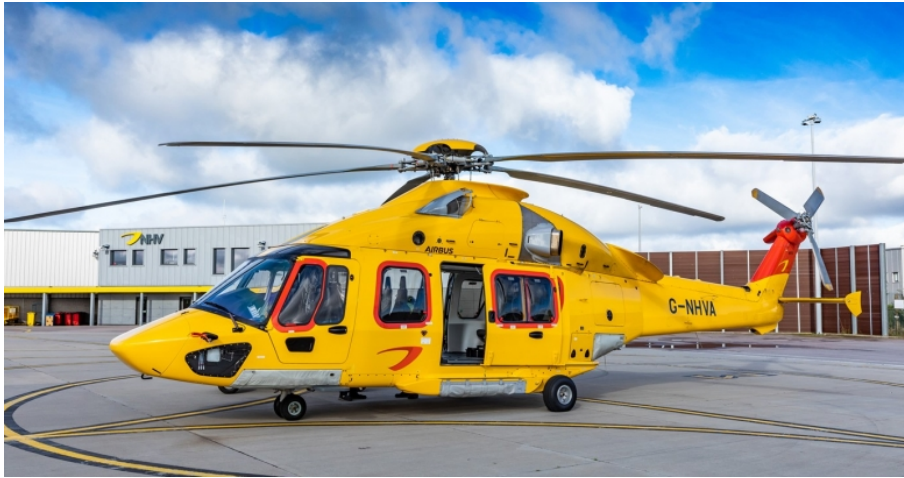
Figure 5.1: Airbus Helicopters H175 with the fairingless rotor head serving as the basis for the RACER rotor head [24].
