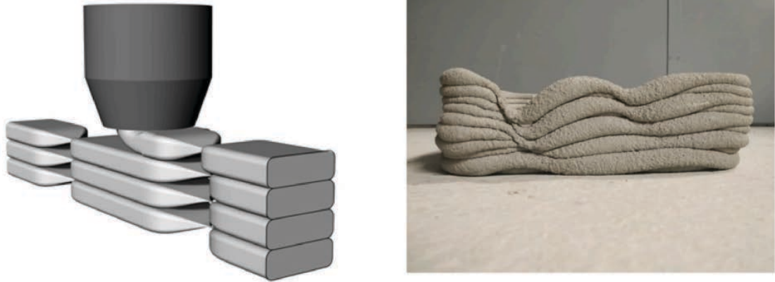
Figure 2.8: Longitudinal tearing at higher speed rate ( V^* ) above the bounding condition (CARNEAU et al., 2022)
