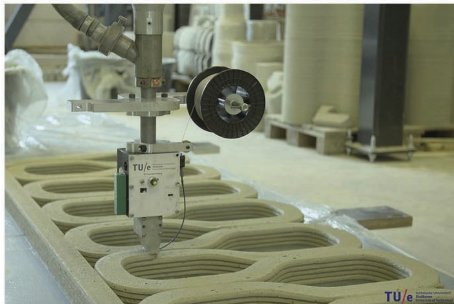
Figure 2.2: Extrusion Method at Eindhoven University of Technology (PAOLINI et al., 2019)
