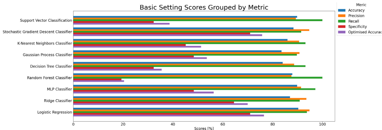
Fig. 3. Comparison of the performance of the standard models of the Scikit-learn library grouped by the metrics accuracy (blue), precision (orange), recall (green), specificity (red) and optimised accuracy (purple). (For interpretation of the references to colour in this figure legend, the reader is referred to the web version of this article.)
