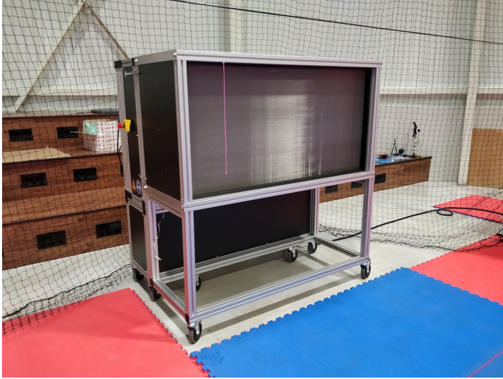
Figure 6.3: WindShape, wind generator located inside ENAC's indoor flight facility.
