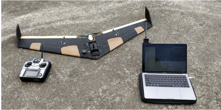
Figure 7.1: Complete flight test system for fixed wing platform.
