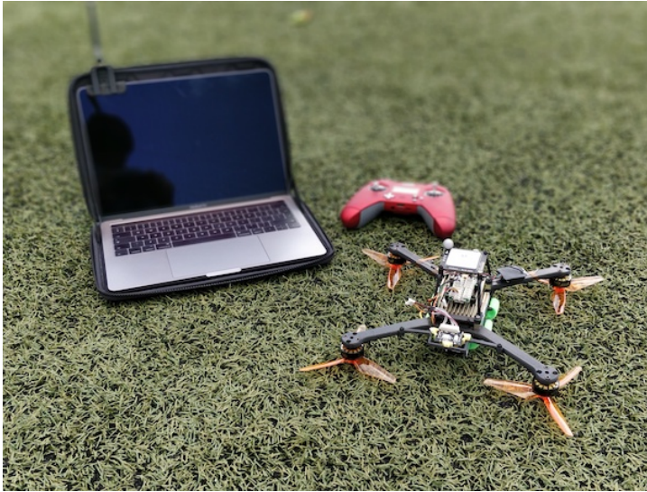
Figure 6.12: Ground control station and the outdoor quad-rotor.
