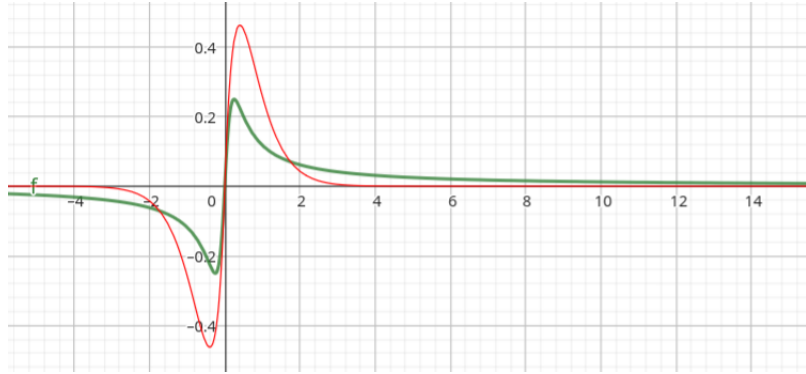
Figure 2.4.: Debye (green curve) and Ohmic (red curve) spectral densities
