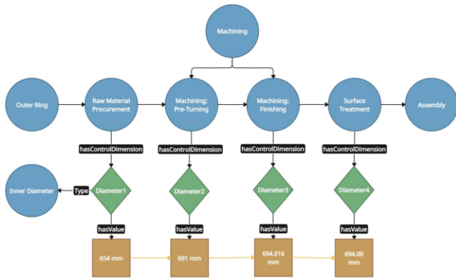
Fig. 5. Taxonomical structure to show the critical dimensions of the different processes for the outer ring stated in the control plan.
