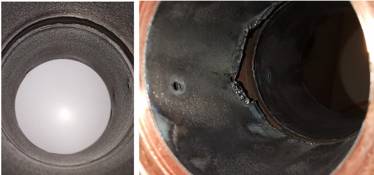
(a) Metallic TBC crack condition before
