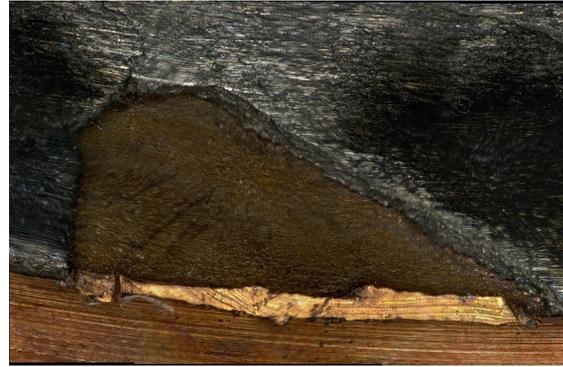
(b) Metallic TBC delamination condition after
