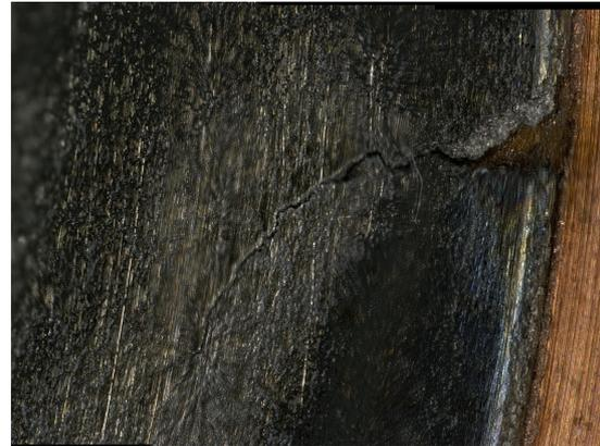
(b) Metallic TBC crack condition at outlet after
