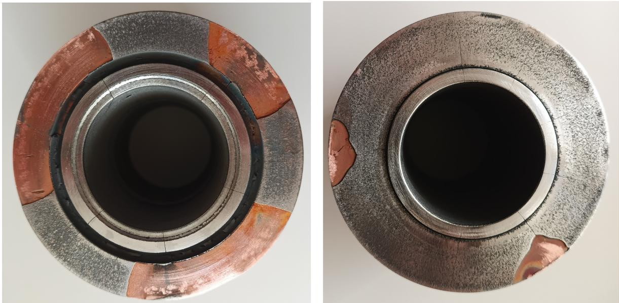
(a) Metallic TBC condition of outlet before post-processing
