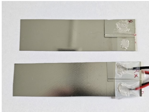
Fig. 10. PEI samples with PVDF-TrFE and electrodes on both sides. (top) Coupon 8, mirror side (bottom) Coupon 2, back side.
