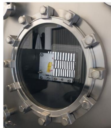
Figure 6 Experimental setup for thermal stability test. When samples are heated uniformly by the radiative source in vacuum, the camera and screen setup can detect small changes in angle. The setup is angled to avoid reflections in the chamber viewport.
