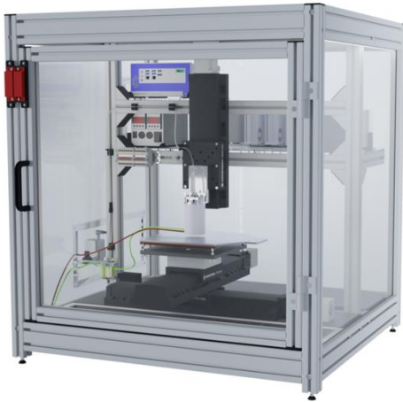
Figure 9: Fully assembled platform configured for flat MEW. A) Rendering of the MEW platform with iPC and the two-zone temperature controller located in the rear left. The Z-axis carrying the print head was mounted on the aluminum frame portal and the X-Y cross-table with collector assembly was mounted onto the base frames of the housing. B) Photograph of the fully assembled MEW platform showing also the high voltage power supply and the operator screen on the left of the system (scale bar 10 cm).
