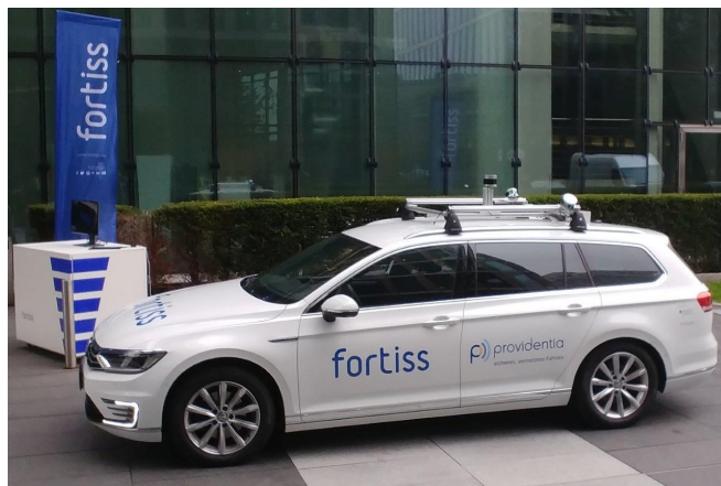
Fig. 1. Fortuna: fortiss' modified Passat GTE with extended sensors and hardware. It is equipped with a prototypical 5G solution to communicate with the intelligent infrastructure of the PROVIDENTIA test field.
