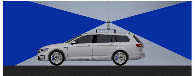
Fig. 4. CAD illustration of the field of view of the central roof lidar (side view). Occlusion effects at the hood are omitted in this illustration.
