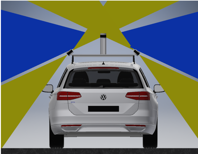
Fig. 5. CAD illustration of the field of view of the lidars (rear view).
