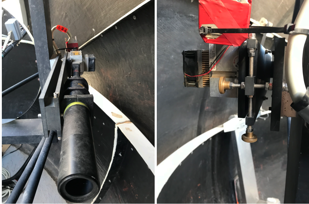
Figure A.4: Images of the old laser mount. The full setup from the front (left) and the screws used for the alignment of the plates (right).
