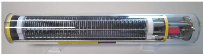
Figure 3.1: Internal part of an ionization chamber (IC) beam loss monitor (BLM) showing the electrodes. The cables to the read-out electronics are located on the right part (fig. from ref. [45]).
