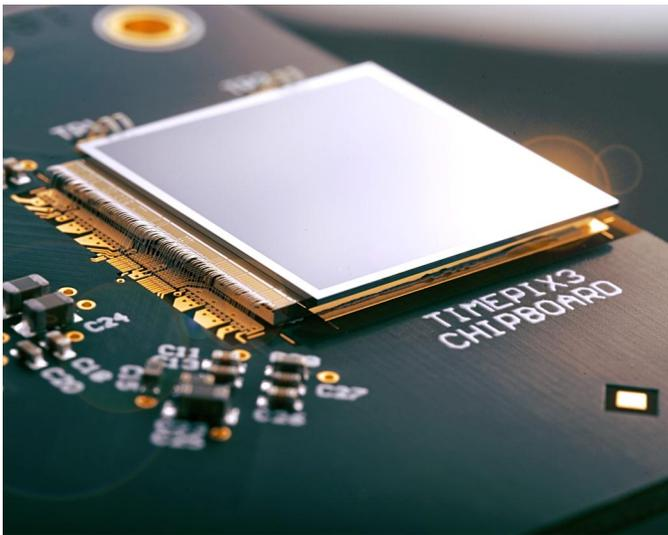
Figure 8.8: Timepix3 chip (fig. from ref. [162]).
