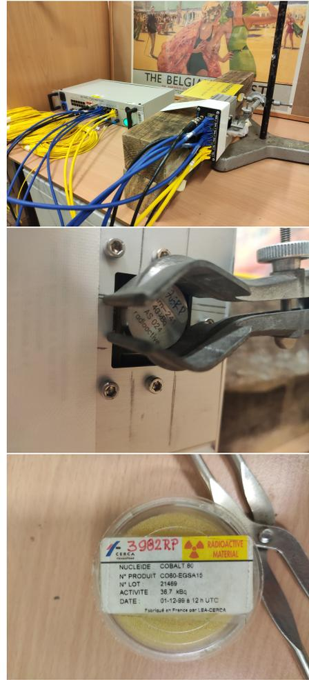
Figure 9.6: Timepix3 radiation monitor, as (top) installed in the CALLAB hall, with (centre) the  $^{241}\text{Am}$  source at 12 mm, and the (bottom)  $^{60}\text{Co}$  source.
